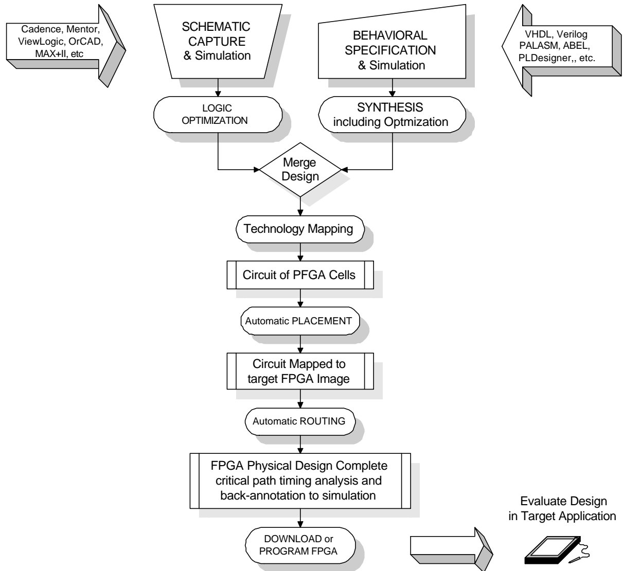
Figure 21. Typical CAD System Design Flow for FPGAs
