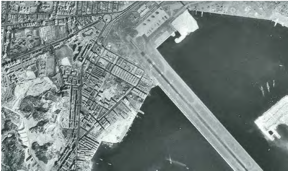
Figure A15 An aerial photographs showing the Sacred Hill levelled in 1964 and the mullah was filled up for construction of the new runway. (Source: Empson 1992)
