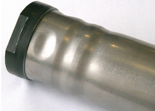
Fig. 9: EMPT crimping of a steel truck wing holder
