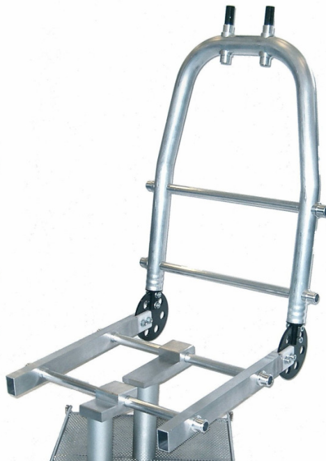
Fig. 10: EMPT crimping of dissimilar materials for lightweight seat structures of cars and aircraft
