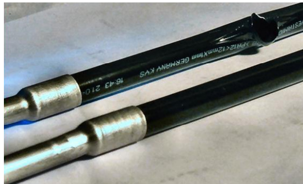
Fig. 8: EMPT crimping of steel fittings onto rubber hoses
