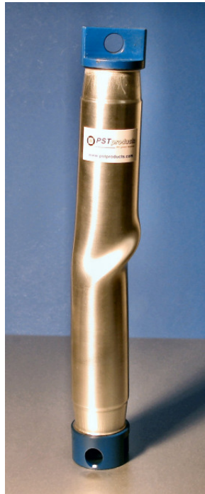
Fig. 13: EMPT welding of steel end pieces into a lightweight aluminum drive shaft
