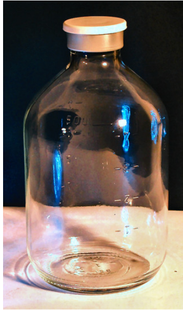
Fig. 11: EMPT crimping of a sterile aluminum lid onto a pharmaceutical glass bottle
