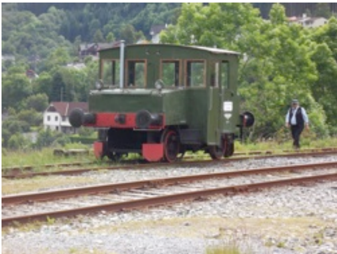
A diesel engine that was used to move train cars around and hook them to the steam engine.
