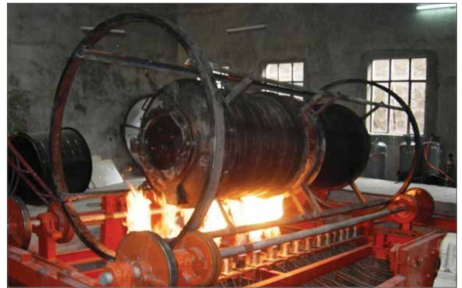
Figure 5b: Open Flame “Rock and Roll” Rotational Moulding Machine
