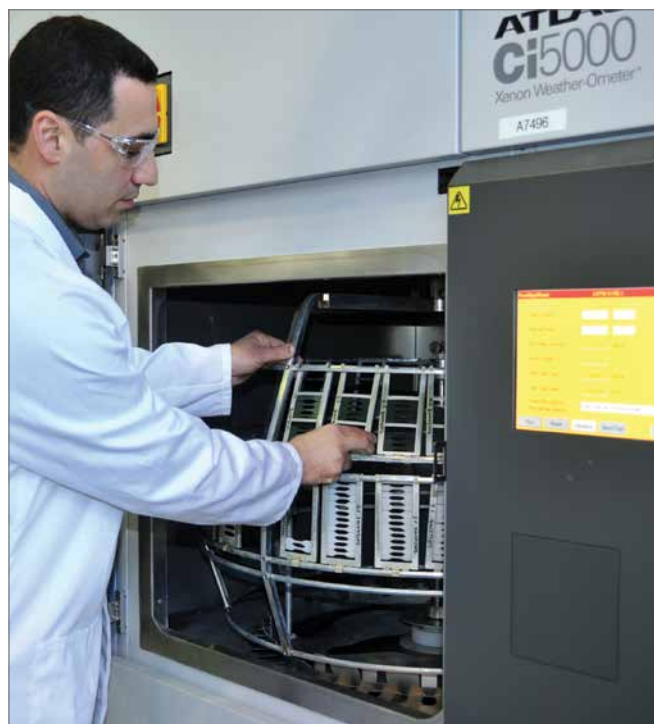
Figure 2: UV performance testing to >20,000 hours against AS/NZS 4766
