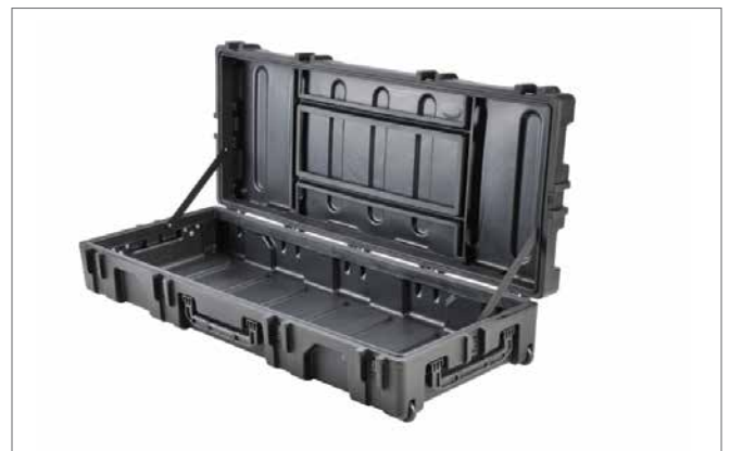
Figure 11: Rotomoulded Case with Large Flat Sides – Moulded Ribs Minimise Distortion and Warp
