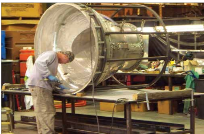
Figure 6: Preparation of an Aluminium Rotomould to Ensure a High Quality Internal Surface Finish
