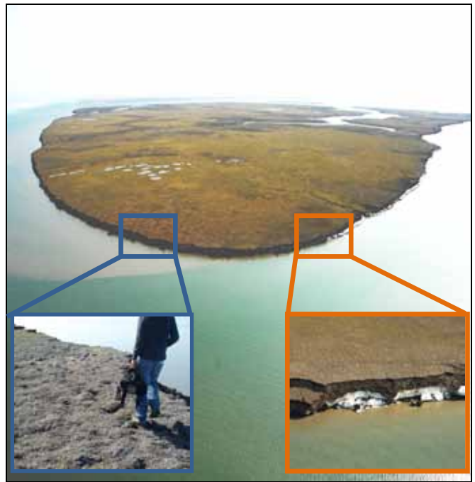
This south-looking view shows the northern tip of Baillie Islands, the farthest north point on the Northwest Territories mainland. The headlands are actively eroding as underlying permafrost thaws (white ice lenses in right-hand inset image), waves undercut the bank, and salt spray from storm surges kills the bankside vegetation (left-hand inset image [ photo credit: Suzanne Carrière ]).
