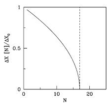
Fig. 3. Plot of the (normalized) distance between two successive collisions  $\Delta X[N]/\Delta X_0$  as a function of the number of bounces N. The initial velocity is  $V_{x0} = 8 \text{ m s}^{-1}$ , corresponding to  $N_c = 17$  (using the same values for the parameters as those given in the text). The vertical dashed line indicates that  $N_c = 17$ .
