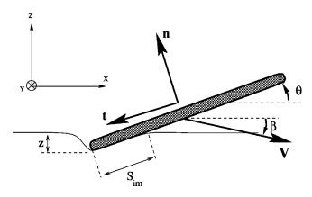
Fig. 1. Schematic view of the collisional process of a flat stone encountering a water surface. The stone has a velocity V, with an incidence angle  $\beta$ , while  $\theta$  is the tilt angle of the stone. The immersed area  $S_{im}$  represents the area of the stone in contact with the water surface. The depth of the immersed edge is z.
