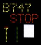
f) Finally the aircraft is perfectly parked at the stop position, and perfectly centered.
