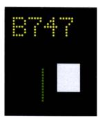
a) In this picture the aircraft is at a distance greater than 30 meters from the parking position and is directly at the center line.
