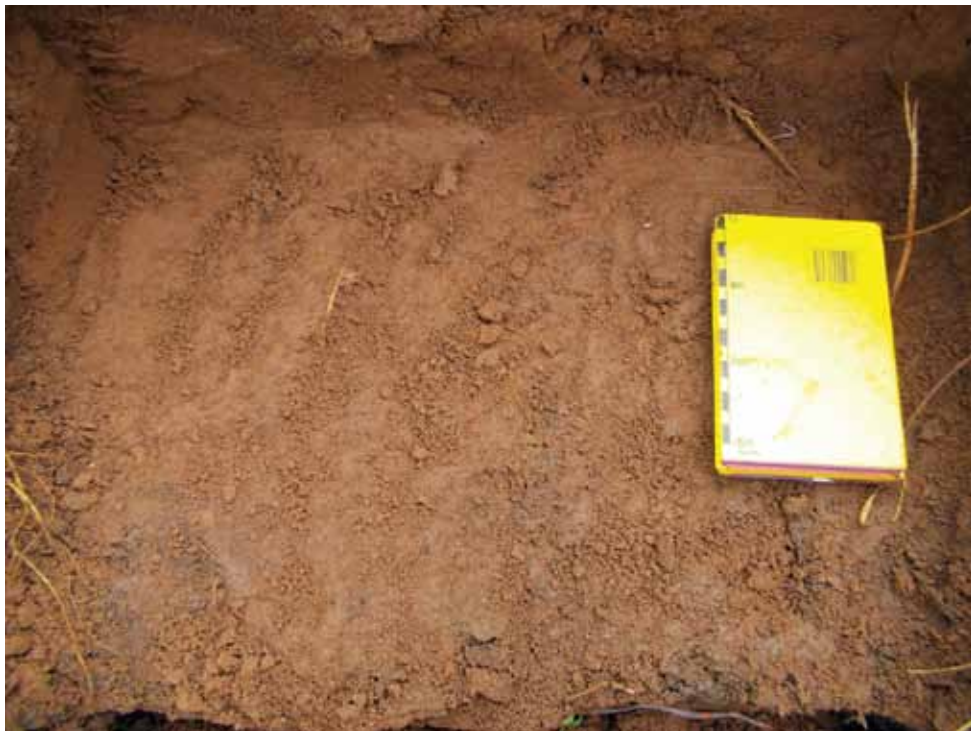
Figure 3-3: Sandy silt (0.40-3.00mbgl) as exposed in east facing section in bank of the River Chew.
