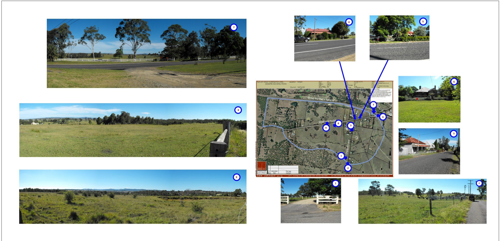
Figure 2.13 Photographic record of site survey showing location plan and orientation of photographs. Photographs by Sue Singleton.
