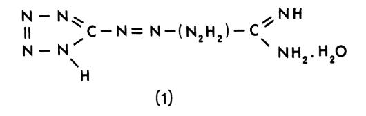
Hermetically-sealed extended-life detonators have been developed to protect lead azide from hydrolysis by atmospheric water vapour and reaction with other incompatible gases. It has been proposed to develop similar sealed caps containing tetrazene in admixture with other substances including lead azide. It was therefore initially necessary to establish whether gas evolution accompanied thermal decomposition of tetrazene during storage,
