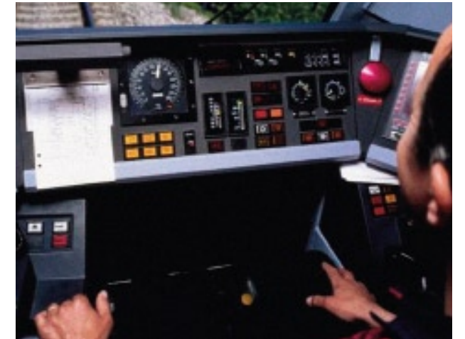
Signalling, EBI Drive 50 , Driver Assistance System
