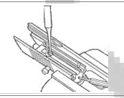
Hold the slide bottom side up in a vise. Depress the firing pin lock (9) with a punch and use a long thin punch from the front to push the firing pin lock and spring are removed, drive out the extractor pin (2), and remove extractor (6), extractor spring (5), and cartridge indicator (3).
