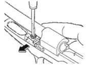
Push the takedown catch all the way to the left, and unscrew the takedown catch screw (34). In doing this, a screwdriver with a thin shank is required to clear the barrel. After removing the screw, shake out the catch and sprig to the right. The hold-open latch and ejector (12) and latch spring (11) can be removed by driving out the hold-open hinge pin (13) to the left. Do not remove these unless necessary.
