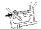
Before attempting disassembly of the lock mechanism, remove the grip screw (15) and grips (14) (27). Then carefully clamp the receiver (41) in a vise with padded jaws. Place a thin metal bar against the bottom of the spring retainer (26), and push on the bar until the retainer is free of the receiver. then ease the bar back to original position and remove the hammer spring (25) from the hammer strut (24).
