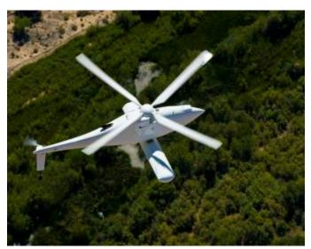
conventional technology. The A160T's unique optimum speed rotor (OSR) system allows the blade RPM to be tailored to flight conditions to significantly improve engine efficiency. The A160T has demonstrated intelligence, surveillance, and reconnaissance (ISR), cargo resupply and high-endurance capabilities and is in production.
