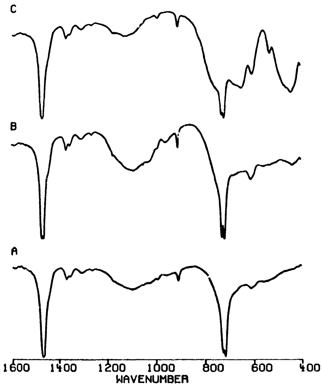
Figure 48. Mid IR of Sb_2S_5 (A) 400°C in Air; (B) 525°C in Air; (C) 700°C in Air.
