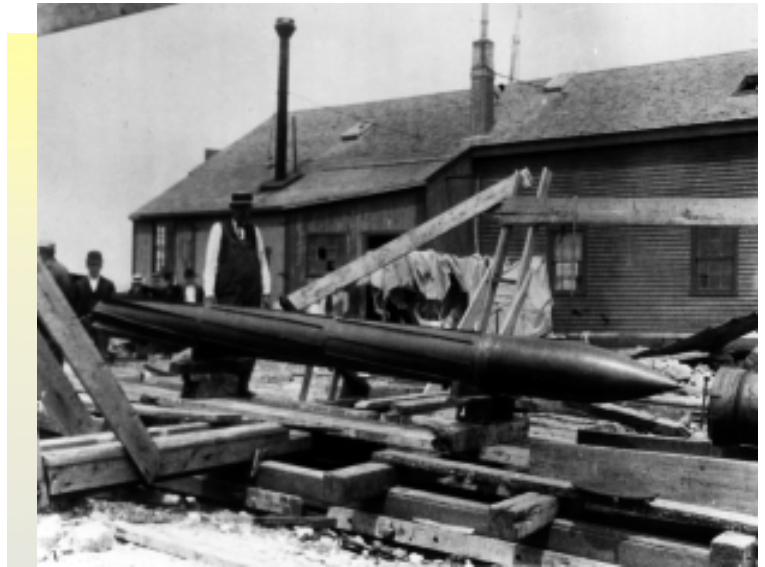
The Cunningham Rocket Torpedo (aft end of the torpedo appears at far right) and its inventor, Patrick Cunningham, are shown in this photo taken at New Bedford, Mass., in July 1893. Lack of accuracy and wide variations in speed kept the Cunningham and other early rocket torpedoes in the experimental stages.
