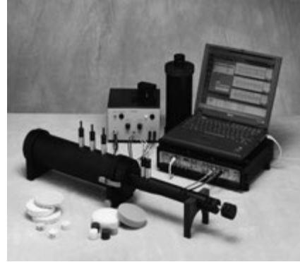
Figure 2. 3560 C type multifunctional analyser of PULSE system and type 4206 impedance tube
