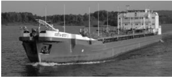
Figure 5. 5000 t river tanker created on the basis of the type "Volzhsky" built-up dry cargo vessel
