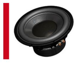
Two new very long stroke subwoofers also arrive with a unique price/performance ratio. The 26W/4558-00 and 30W/4558-00 both feature matching passive radiators. The 26- (10") and 30cm (12") subwoofers, respectively, have very high excursion capabilities (X-max 56mm), frequency performance below 20Hz, high power handling, and are optimised for compact cabinet volumes. They are suitable for both active as well as passive constructions.
