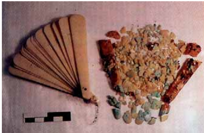
FIGURE 28: An example of how similar artefacts, made by celluloid ( an artificial plastics ), may present different degree of degradation. Left , Fan ( 1920 ) with a good state of conservation. Right , Fan completely disintegrated [39].
