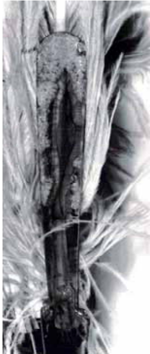
FIGURE 8: It is illustrated the degradation of cellulose nitrate observed on the handle of the Beatrice Lillie fan , made in celluloid ( Theatre Museum collection of the Victoria & Albert Museum, London ) [6].
