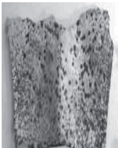
FIGURE 21: Degradation effects of bacterium colonization, Nocardia sp. Strain-MBR, on samples of natural rubber-latex gloves [35].
