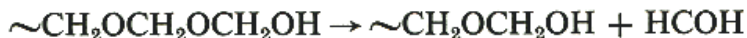
FIGURE 17: Depropagation reaction from chain ends in the case of polyoxymethylene ( polyformaldehyde ). Monomer products are formed [9].
