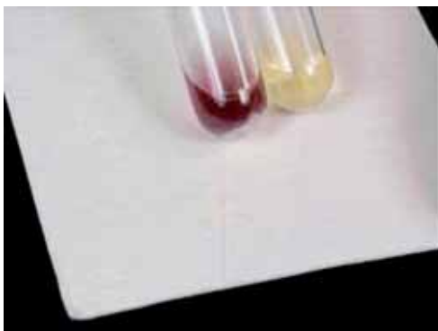
FIGURE 31: The hydroxylamine hydrochloride test used to identify cellulose acetate in artefacts.
