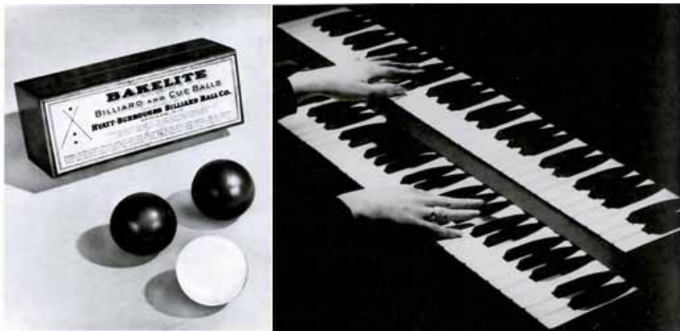
FIGURE 14: Left , billiard balls made in bakelite [9]. Right , styrene-acrylonitrile ( SAN ) and acrylonitrile-butadiene-styrene ( ABS ) resins replaced ebony and ivory in making organ keys [26].
