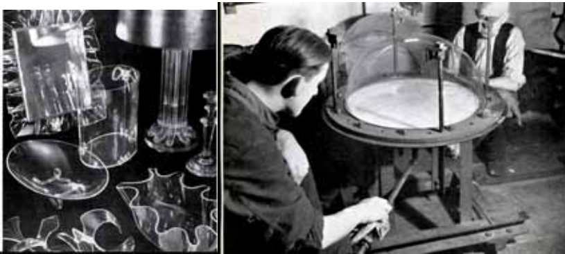
FIGURA 15: Left , decorative artefacts made in PMMA ( year 1940 ) [6]. Right , an aircraft “ gun-sighting ” blown from a sheet of PMMA ( I. C. I. Plastics Division, second world war ) [11].
