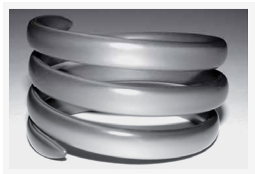
FIGURE 6: shrinkage effects ( see whitened regions ) observed in a cellulose acetate bangle due to plasticiser loss [7].
