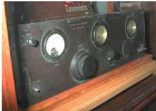
FIGURE 27: The radio-field, kept at the “Museo dell'Arsenale della Marina Militare”, La Spezia”, used during the expedition of the aircraft “ Italia ” to the North Pole. The frontal part is made in hardened rubber.
