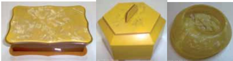
FIGURE 9: Boxes in celluloid belonging to the M. P. Incutti collection ( Naples ) whose state of conservation was investigated in the framework of the project cited in reference [14].
