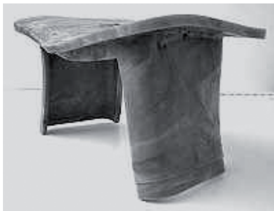
FIGURE 4: Object in cellulose acetate with evidence of distortion due to uneven migration of plasticisers [4].
