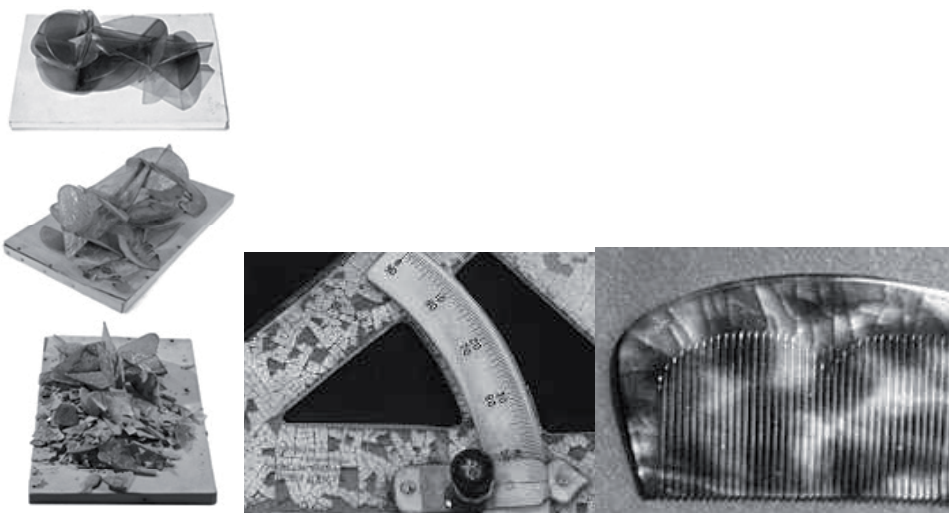
FIGURE 1, left: < The series of images... shows the stages of degradation of Antoine Pevsner's 1923 "Head of a Woman," made of nitrocellulose plastic. Courtesy of the hirshhorn museum; John lee/National Museum of Denmark > [5].
