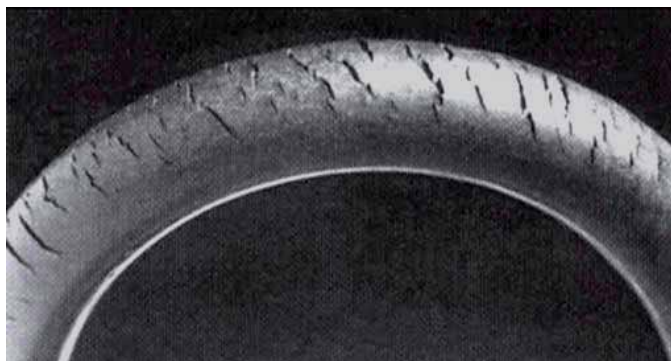
FIGURE 12: Development of cracking structures produced in natural rubber tubing by the exposure to ozone [8].
