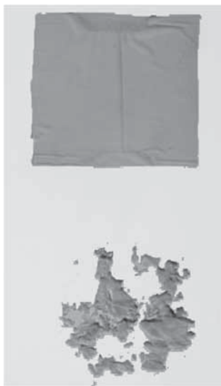
FIGURE 1: Films of linear low density polyethylene. Top , practically undegraded. Bottom , fragmented following severe molecular and mechanical degradation, thus suitable to be biodegraded by microorganisms.
