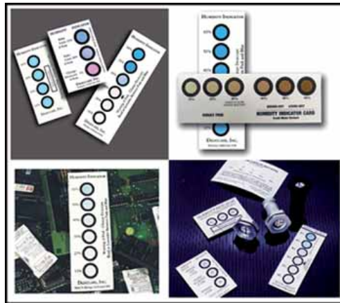
FIGURE 20: Exemplars of color changing “Humidity Indicating Cards” (HIC) used to monitor the humidity content inside an enclosed show case or display cabinet [36].
