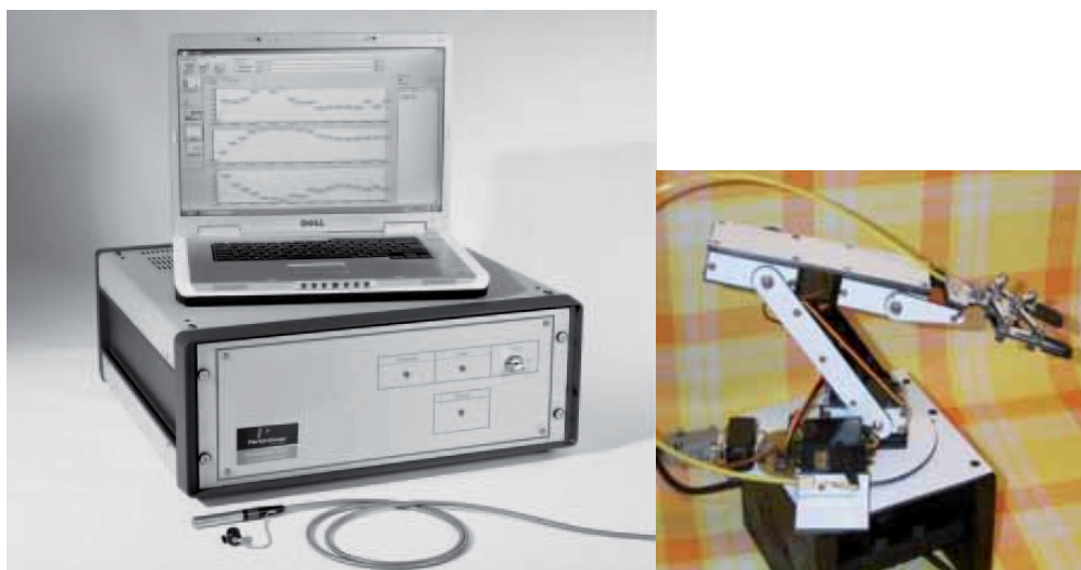
FIGURE 15: A mobile Raman spectrometer equipped with an optical fibre probe that can be positioned on the surface of the sample to be analysed, thus suitable to perform non destructive analysis on plastic artefacts [23].
