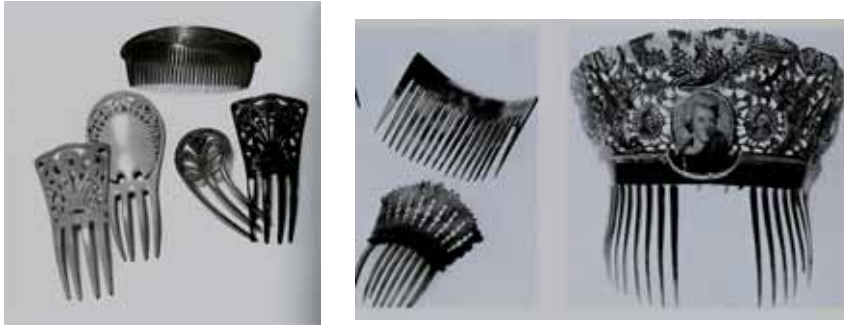
FIGURE 13: Left , combs manufactured in horn, Leominster, Massachusetts, USA, (latest 1800s ) [9]. Right , artistic combs produced in celluloid ( early 1900s ) [9].
