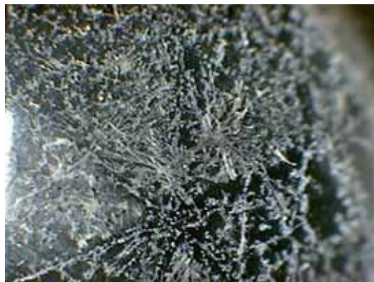
FIGURE 3: Crystal like growths caused by additives, observed on the surfaces of cellulose nitrate or cellulose acetate objects [3].
