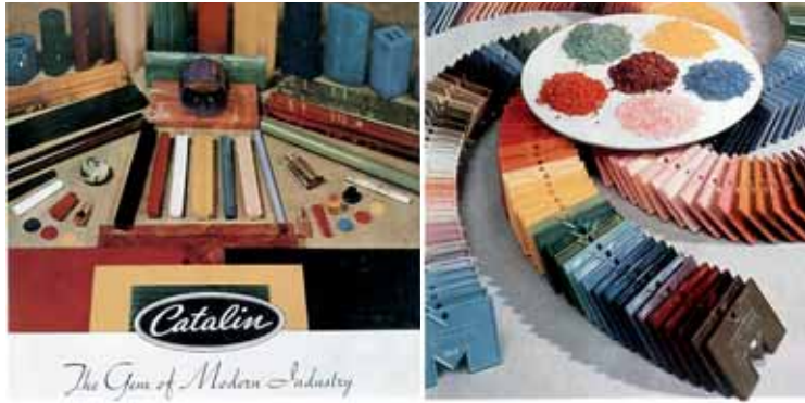
FIGURE 1: The development of new plastics and pigments led to the production of materials having a wide variety of colors. Left , a catalogue ( 1936 ) of the Catalin Company showing “ the colored Gem of the modern industry ” based on phenol-formaldehyde resins. Right , set of samples in poly vinyl acetate with different coloration [6].
