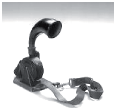
FIGURE 14: Ebonite was also used in the manufacturing of components for telephones (year: 1900 ), Plastics Museum Cannon for the Culture of Plastics [23].
