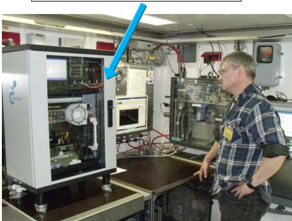
Fig. 4: SubCtech “Ocean Pack” for Water- p\text{CO}_2 underway measurements on RV “Polarstern”, (Images SubCTech)
