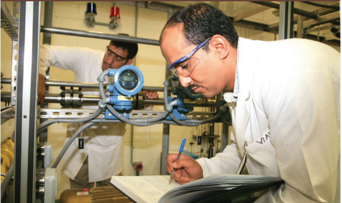
The company's downstream research projects include studying the performance of industrial materials under simulated production conditions. Here, company researchers monitor the progress of a corrosion simulation experiment utilizing a unique corrosion flow loop apparatus.
