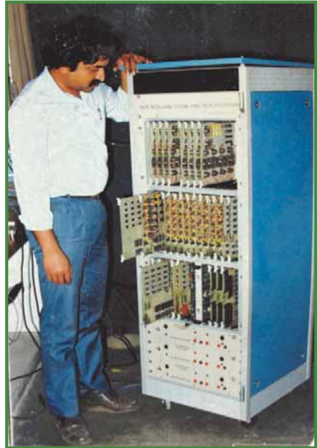
The prototype of the Electronic Interlocking system
