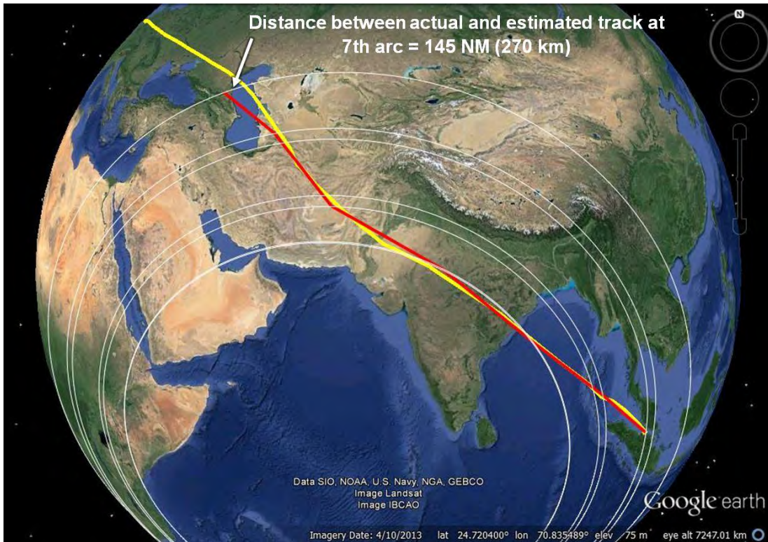
Figure 30: MH021 07 March 2014 - The red path is predicted path from BTO/BFO values; yellow track is the actual aircraft track
