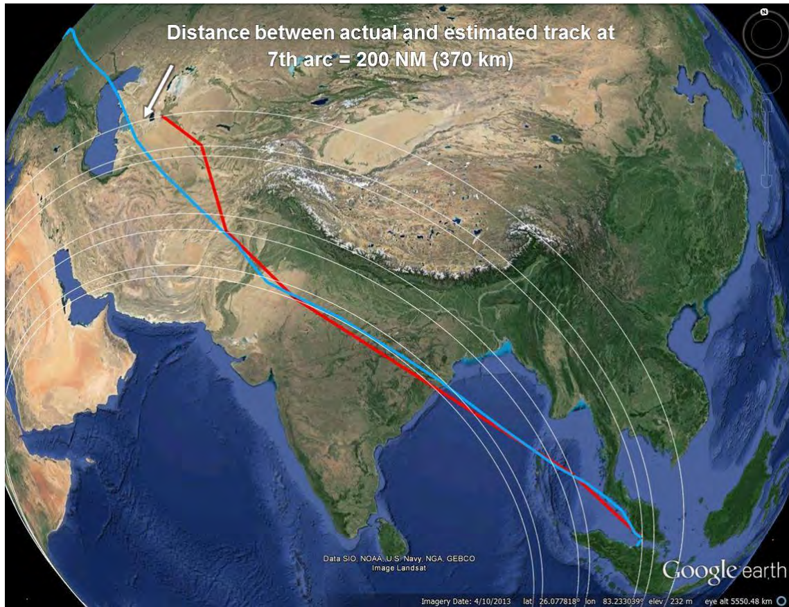
Figure 31: MH009 07 March 2014 - The red path is predicted path from BTO/BFO values; blue track is the actual aircraft track.
