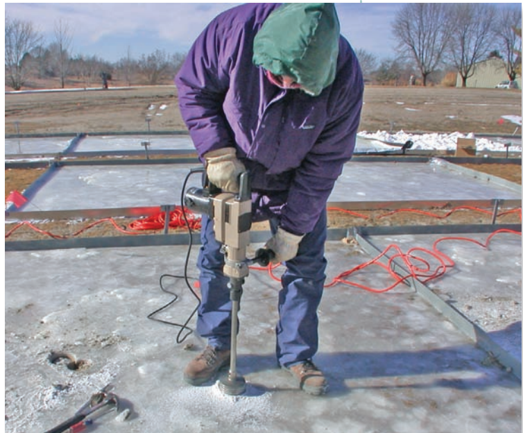
An impact hammer drill was used to sample greens during the winter to determine when the grass actually dies.
