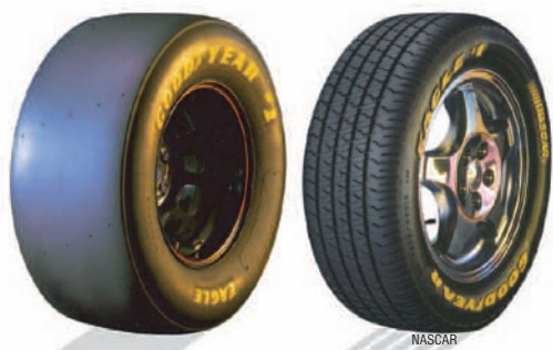
Goodyear Eagle Radial Race Tire Tread Width: 11.5 inches Average Life: 150 mi
