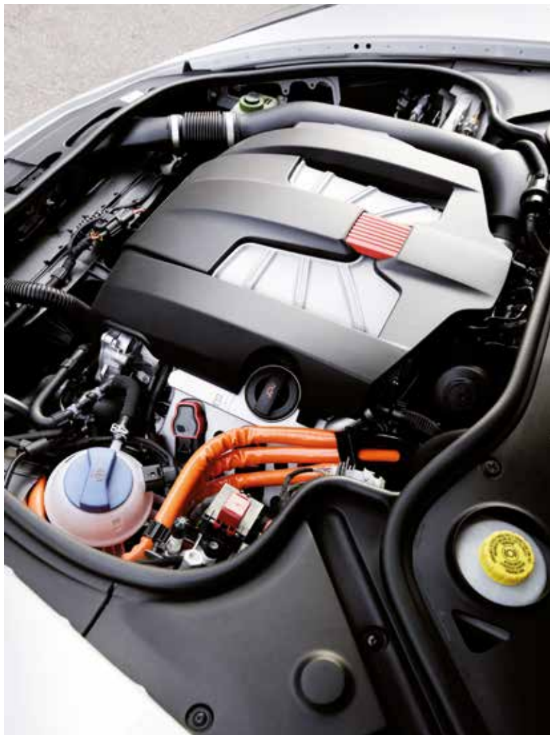
Combustion engine plus electrical motor: Thick cables reveal the presence of a high-voltage system.
