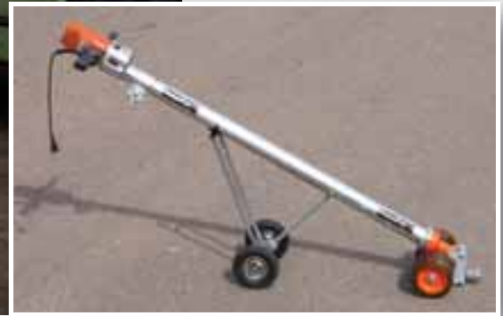
The toe coupling of the PowerCat is attached to a set of skates
