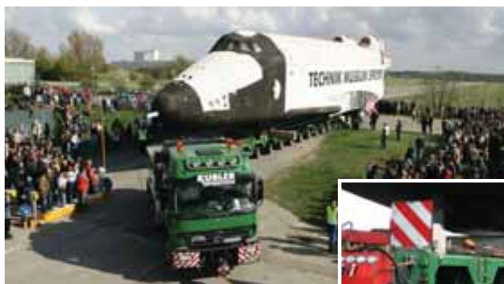
RIGHT: The Buran rolls on land loaded on 16 lines of Scheuerle Intercombi hydraulic modular trailer
