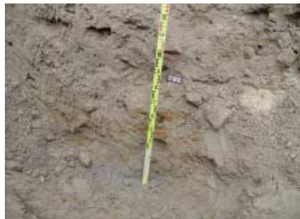
Fig. 6. The two lowest till units in test pit M55 at Portimojärvi, Ranua. A sharp contact between the bluish grey (bottommost) and grey tills are seen at the base of the section at a depth of about seven meters. Iron-stained, brown bands indicate the groundwater level variation. Photo P. Sarala.
