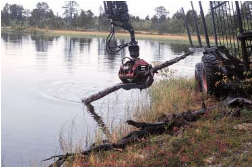
Fig. 2. Sampling with loading crane and log grips.
