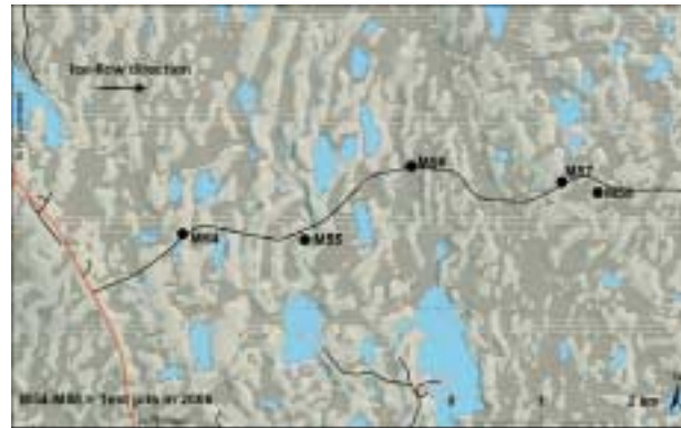
Fig. 5. Part of the ribbed moraine field near the Portimojärvi village in Ranua. Test pits dug during 2005 are marked as M54–M58. Digital elevation model, topographic features and roads © National Land Survey of Finland, permission number 26/LA/07.
