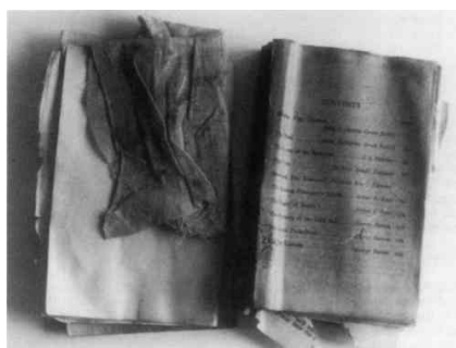
FIGURE 4: Untreated book after 4 months of immersion in water followed by 3 months of storage while still wet [11].
