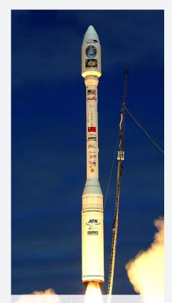
The Minotaur-C launch vehicle is a groundlaunched variant of Orbital's highly successful Pegasus air-launched space booster.
