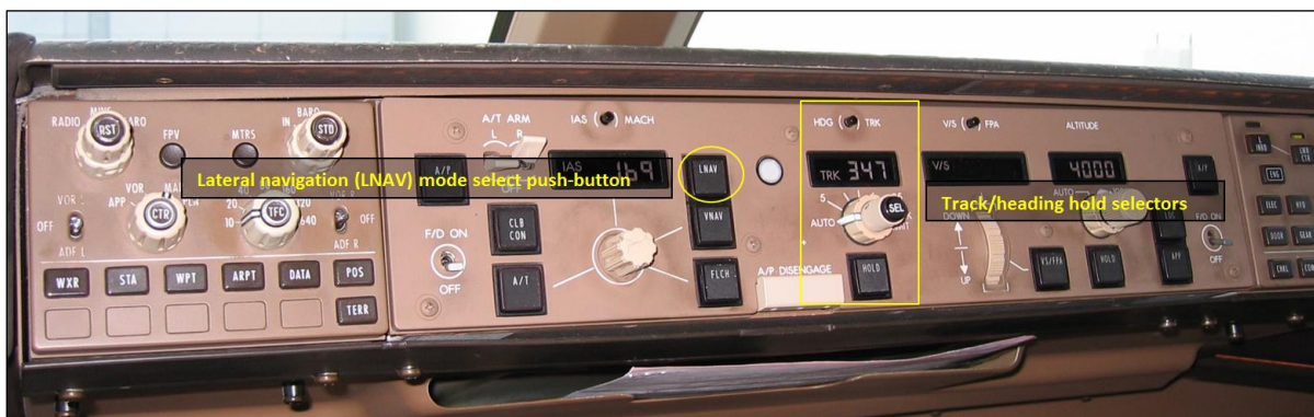
Figure 33: B777 LNAV mode and track/ heading hold selectors
