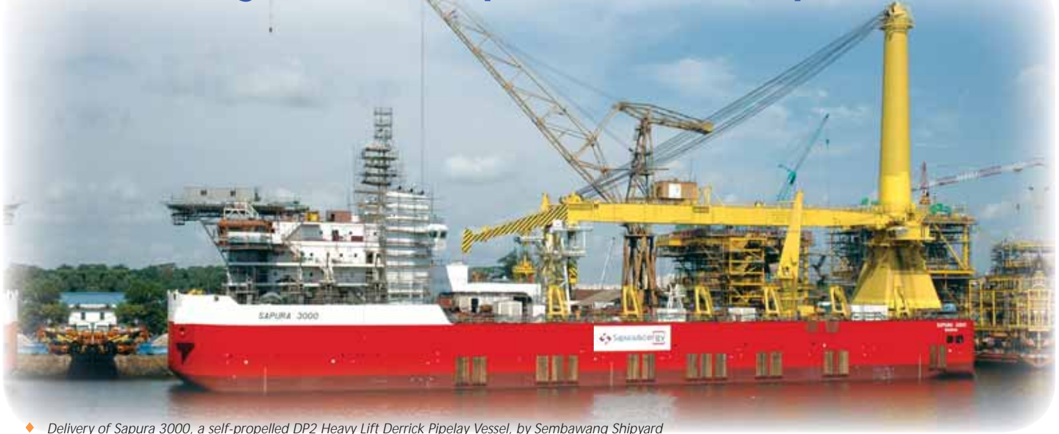
◆ Delivery of Sapura 3000, a self-propelled DP2 Heavy Lift Derrick Pipelay Vessel, by Sembawang Shipyard
