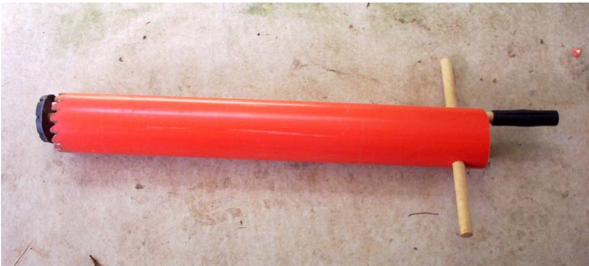
Fig. 3. The pipe sampler used during this survey for quantitative benthic sampling.
