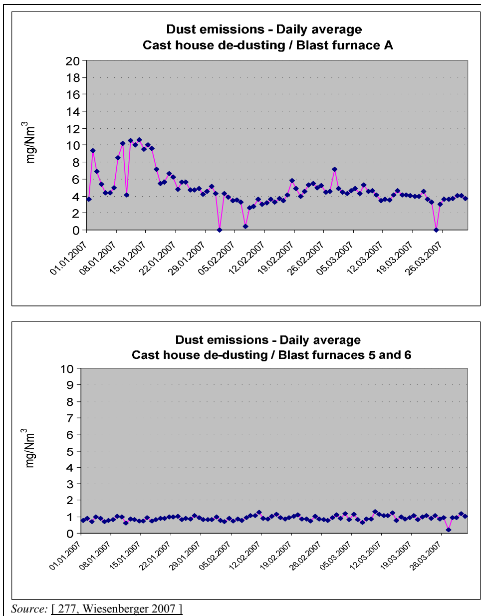
Figure 6.14: Daily average emission values of cast house dedusting systems at tap holes and runners of blast furnaces at Voestalpine, Linz, Austria
