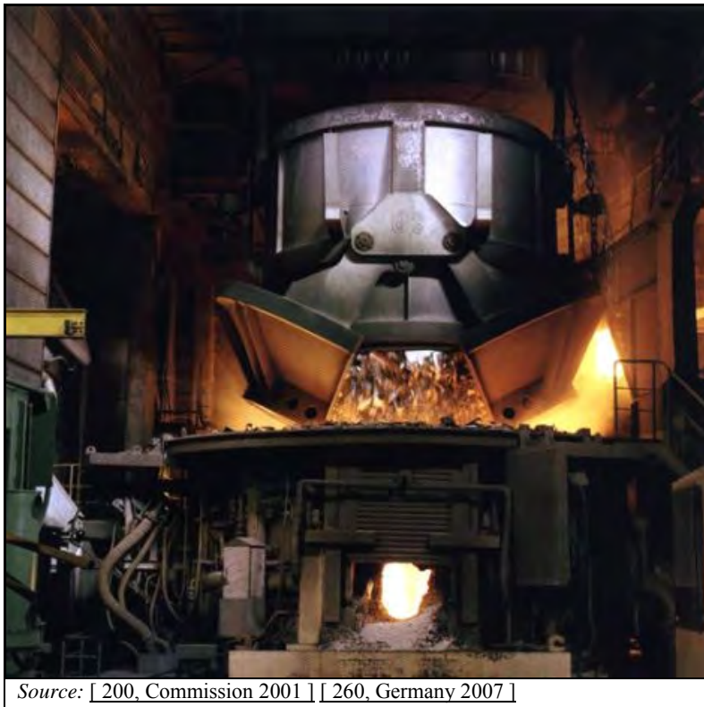
Figure 8.2: Electric arc furnace charging
