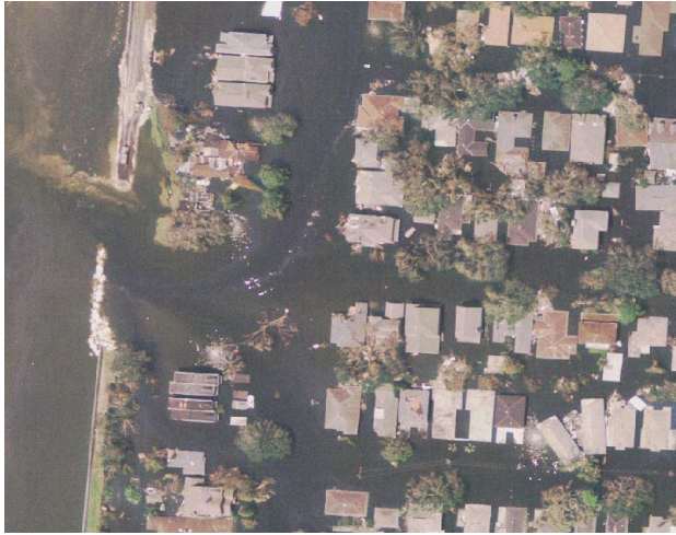
Left: Sandbags could not close the levee breach in New Orleans' Metairie Relief Outfall Canal. Flooding reached roofs, pushed buildings off foundations, and created a maze of fallen trees. Right: Bayou St. John snakes between the New Orleans Museum of Art and Saint Louis Cemetery Number 3. Flood waters engulfed the cemetery and City Park, but high ground spared the museum.
