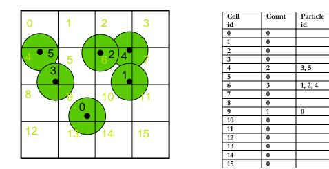
Figure 2 – Uniform Grid using Atomics
