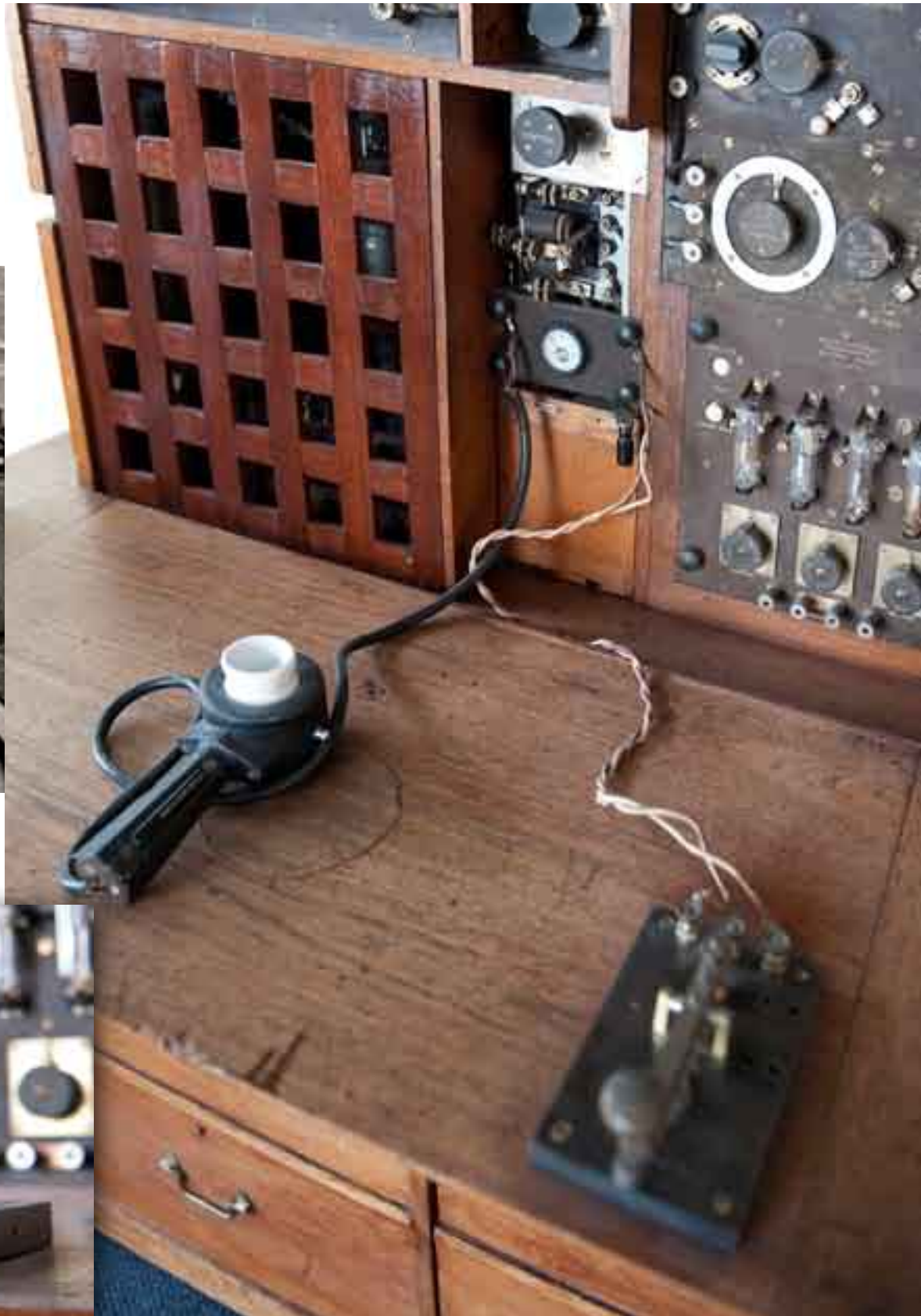
> Radio telephone microphone and morse key of a Marconi mobile radiostation of the 1920s.
