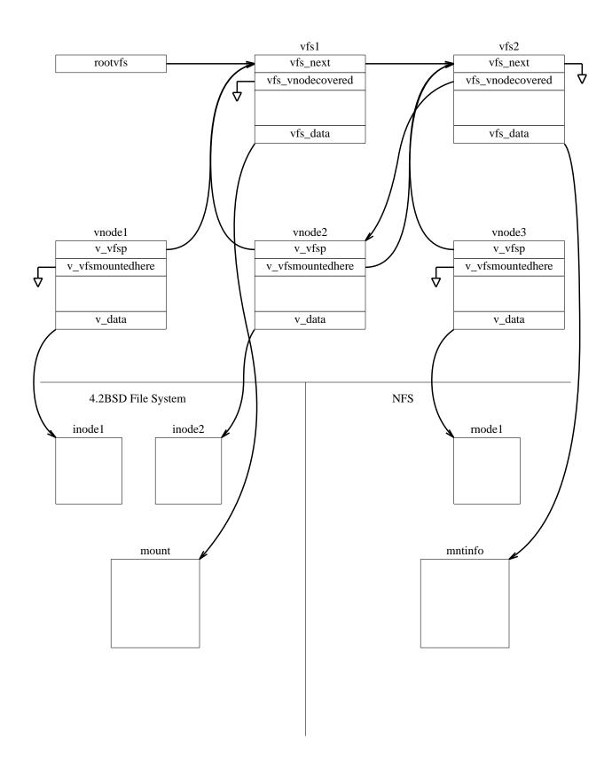
Figure 3. Example vnode layer object interconnection
