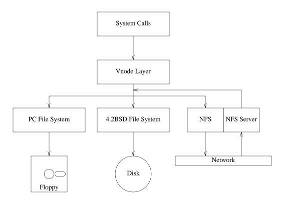
Figure 1. Vnode architecture block diagram
