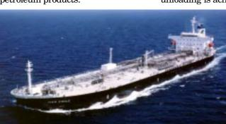
The tanker employs double hull construction for the ship sides and bottom, complying with the latest requirements of MARPOL. Cargo oil tanks use the segregation system to load four types of cargoes simultaneously. Efficient cargo loading and unloading is achieved using the self-
