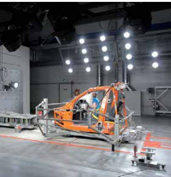
The first servo-hydraulic catapult-sled unit in Europe. Photos: Frank Reichel
