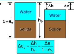
• In the above equation,  $\Delta e$  is the change in void ratio due to the loading increment and  $e_0$  is the void ratio of the soil sample before the application of the loading increment.
