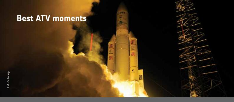
↑ Launch. A launch is one the most challenging moments in a mission. ATVs are launched into orbit from Europe's Spaceport in Kourou, French Guiana. ATV *Georges Lemaître* is the heaviest spacecraft to be orbited by any Ariane rocket so far, with a mass of 20 275 kg.
