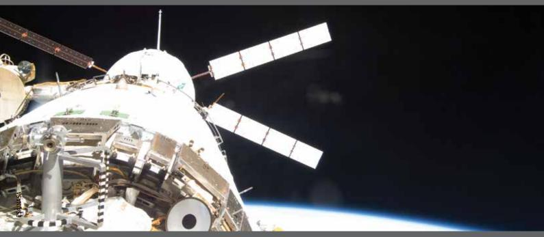
↑ Docking. During the last 250 m until contact with the Space Station, ATV's state-of-the-art automatic rendezvous system employs a videometer's eye-like sensors that analyse laser beams. Despite its mass of about 20 tonnes, the ferry can manoeuvre itself to within a few centimetres.
