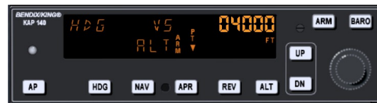
Figure 10.10: Autopilot with altitude armed
