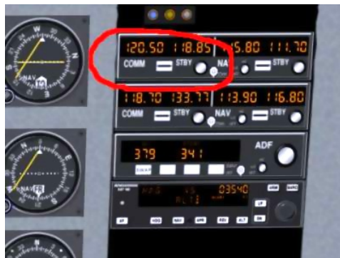
Figure 9.4: The C172 communications stack with COMM1 highlighted
