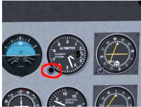
Figure 9.7: Altimeter calibration knob
