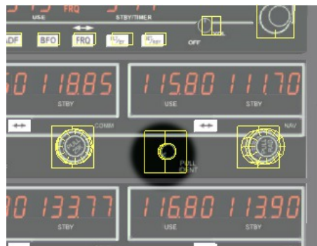
Figure 10.6: Ident volume knob and hot-spots
