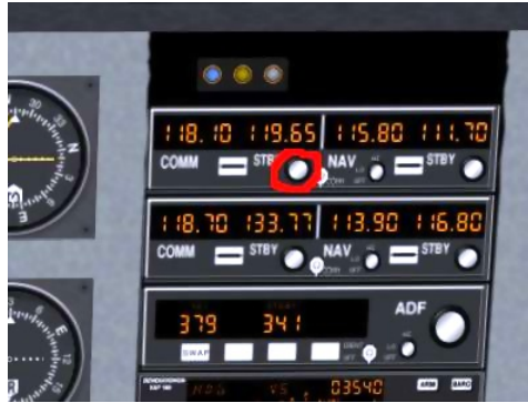
Figure 9.5: COMM1 adjustment knob
