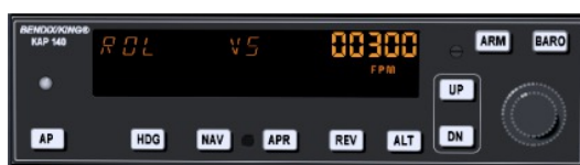
Figure 10.7: Autopilot after engaging
