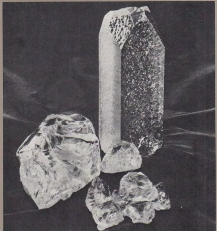
Above—The beautiful quartz crystal standing in the rear is one grown at our Merrimack Valley Works. The pieces in the foreground are nature's handiwork. Both types are used to provide material for electrical filters. Below—President Eisenhower gets nation's 50-millionth telephone from AT&T's Cleo F. Craig.
