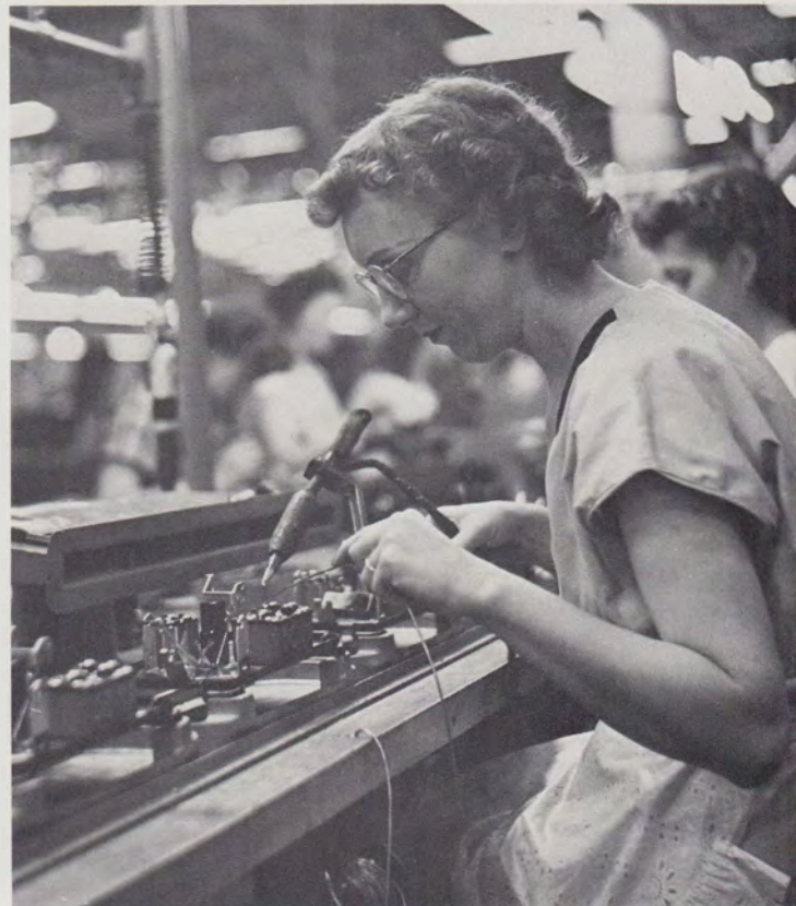
This one wasn't easy — at least not for your editors, who were off by more than a decade. The original caption said she's soldering terminals on the base of the new 500 set which should give you a hint. The place is the Indianapolis Works. The year? 1951.
