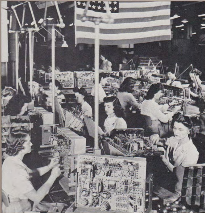
The armed forces needed all kinds of sophisticated communications equipment. This is a carrier telegraphy system, capable of transmitting 12 teletype messages simultaneously, being built for the Signal Corps at Kearny Works.
