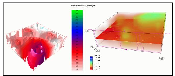
Fig.2 - 3D raster volume representations: The left figure displays isosurfaces representing soil texture distribution (fine sand share) generated by r3.showdspf, the right figure was created by Vis5D (fine sand share, view rotated by 90 degree). The project volume is: 2 km x 2 km x 2 m depth.
