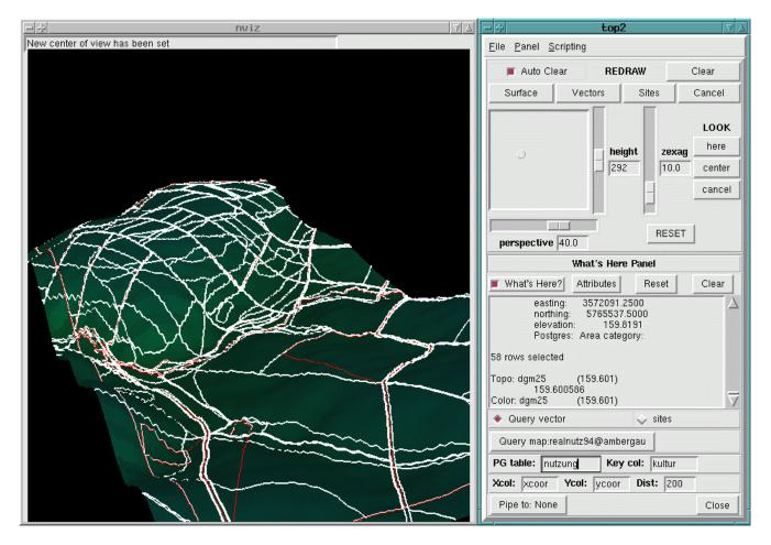
Fig.1 - The NVIZ screen displaying raster and vector data (3D query mode with link to SQL database)
