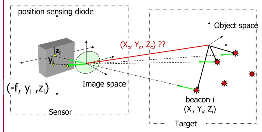
Estimate 6-Dof relative information between the receiver aircraft and the drogue from sensor readings. (Gaussian Least Squares Differential Correction)
