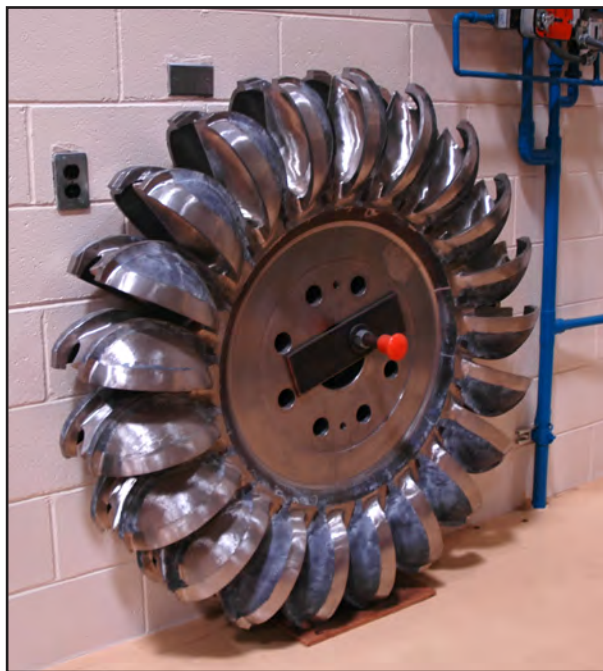
This Pelton impulse turbine (on display in the Betasso Hydro Plant), left, is similar to the one in use at that facility, located in a separate building on the grounds of the Betasso Water Treatment Plant. Pettem photo, 2013
