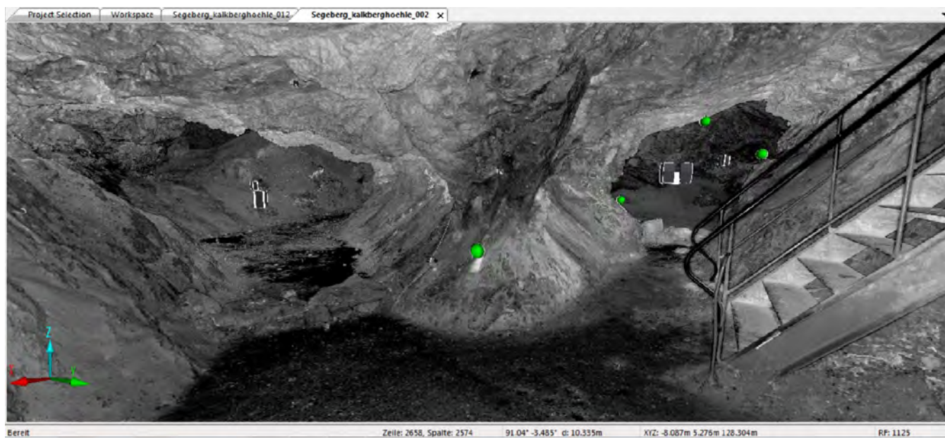
Figure 2. 3D scan of a solutional passage of the Segeberger Kalkberghöhle in anhydrite with typical sloping sidewalls and horizontal ceilings characteristic of a cave created by internal convection.
