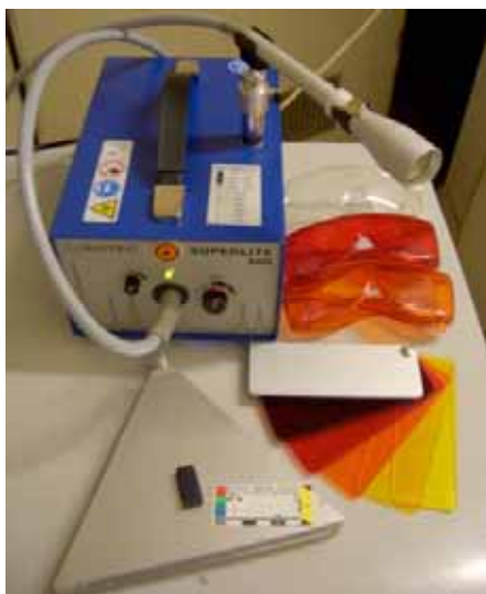
Fig. (2). Lumatec Superlite 400 forensic light source with spot or fan light guide applicator, tree high pass goggles and lorgnette with 5 filters.
