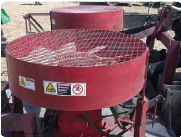
Blowers mounted on slashers can help reduce weed seed spread.
